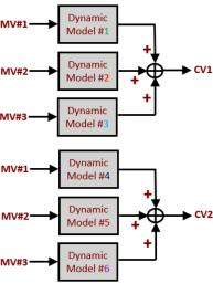
See the six models shown to the left here. PITOPS helps to identify the real open-loop dynamic models after which PITOPS generates model files containing the new and improved MPC models. This functionality of closed-loop data analysis and open-loop dynamic model identification has been hailed as a processcontrol technological breakthrough and is expected to revolutionize the way MPCs are maintained today. This approach can save a lot of time and help to pinpoint the culprit models.
