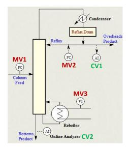
left. There can be six dynamic models for the 3MV – 2CV MPC as shown to the right.
